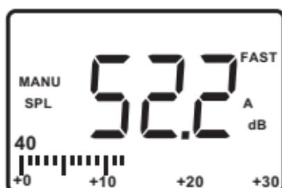
The meter will be able to take readings more quickly, because the unit does not need to first establish the range before displaying the measurement.
