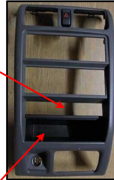
Center Panel (OEM - with Re-Used 1 DIN Compartment and 0.5 DIN Drink Holder)
