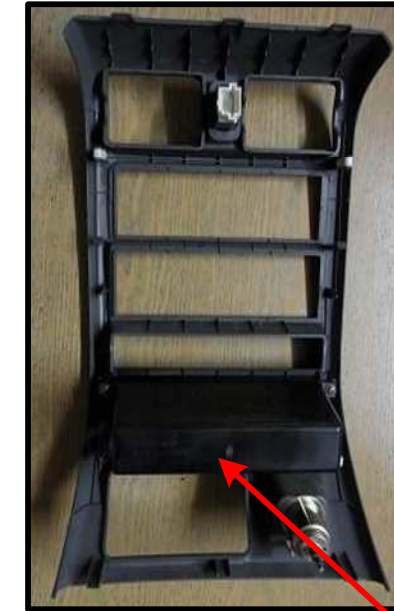
Center Panel (OEM - with Re-Used 1 DIN Compartment and 0.5 DIN Drink Holder)
