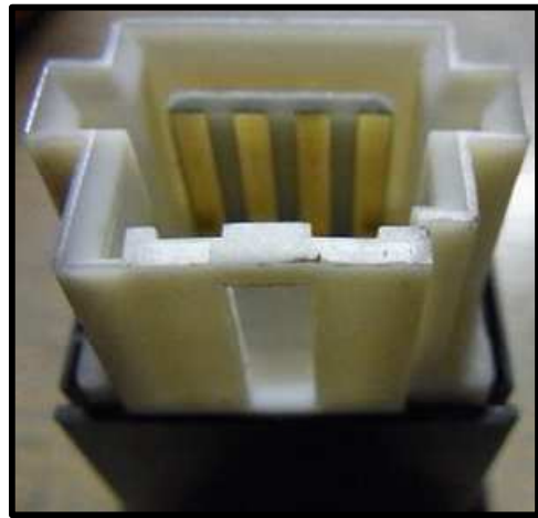
Hazards Switch Socket
