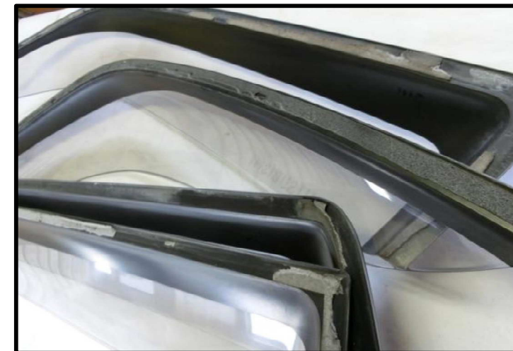
Double-Sided Tape in Bad Condition
