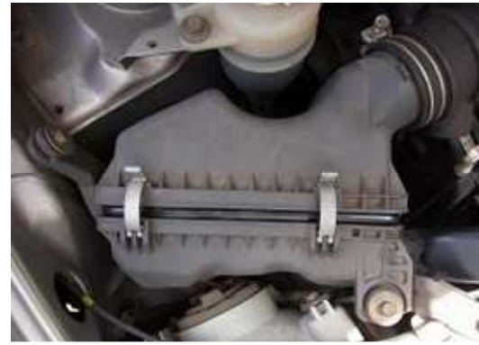
Step-2 Clean away any excessive dirt and grim from the Engine Intake Air Filter Assembly.
