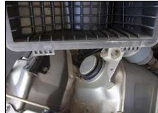
Step-8 Put air filter cover back on, using the two (2) tabs on the bottom as a guide.
