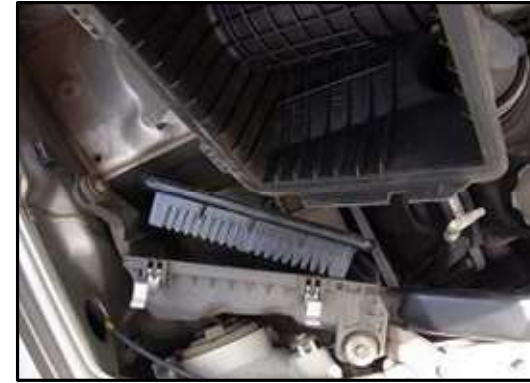
Step-6 Remove old air filter and inspect condition.
