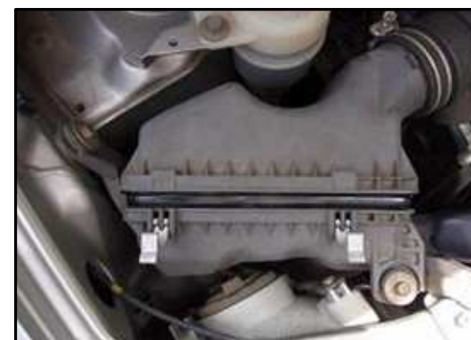
Step-9 Check and ensure that the air filter cover is uniformly seated around filter.
