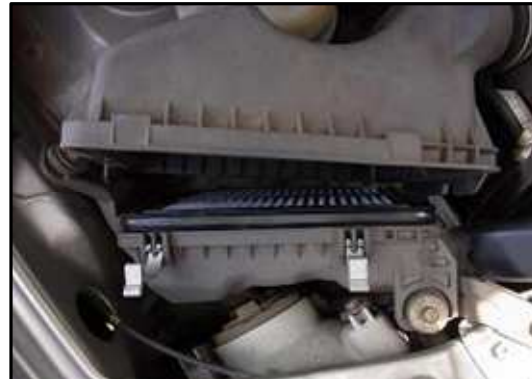
Step-4 Push rear cover with air hose, back away from front cover with Holding Buckles and air filter.
