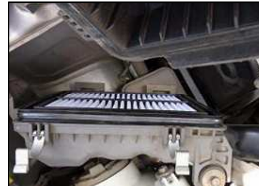
Step-7 "Replace old" or "install new" air filter.
