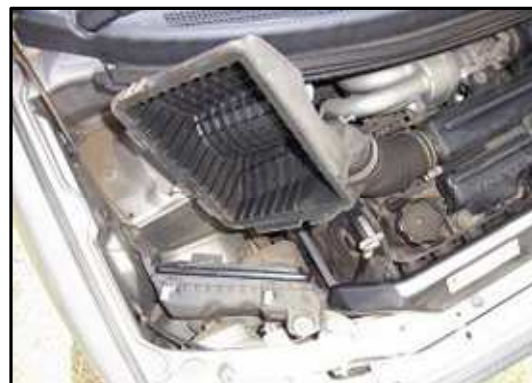
Step-5 Carefully pull up on rear cover and air hose, making sure not to damage air filter.
